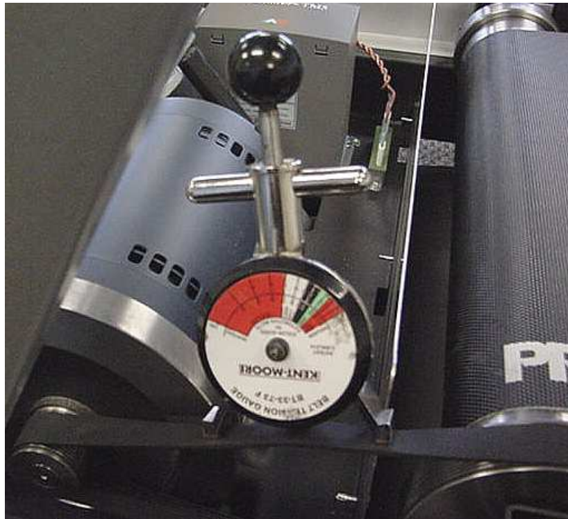
Diagram 4.2 - Drive Belt Tension Gauge
