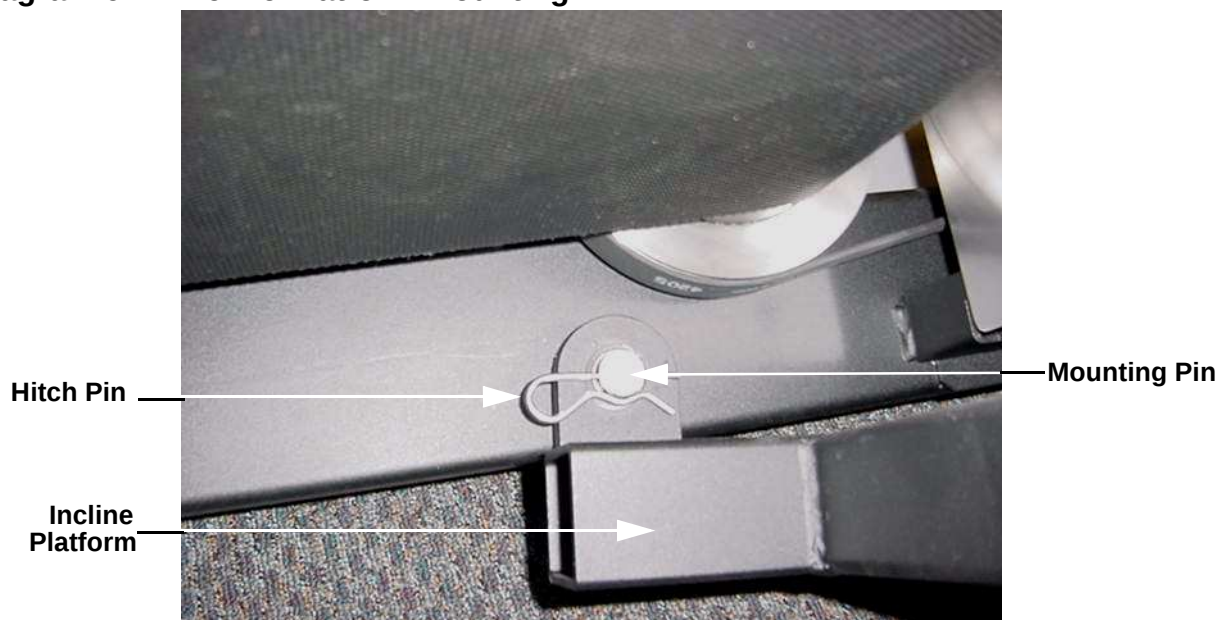
Diagram 6.1 - Incline Platform Mounting
