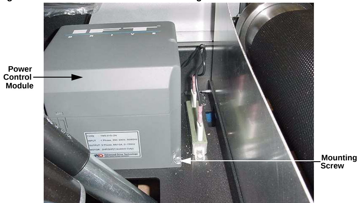
Diagram 6.3 - Power Control Module Mounting
